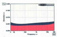
ABOVE: Distortion versus extended frequency from 5Hz-40kHz at 0dBV (left, black; right, red)
