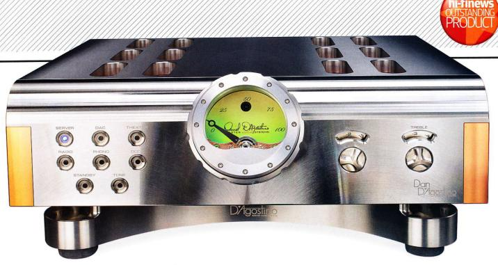
At first glance the Momentum looks like an elaborately sculpted single chassis preamplifier. In fact it's a two-box design, with a substantial linear power supply housed in a slim separate enclosure that forms a base platform upon which the main unit is sited. This is an extremely neat solution. Chunky rubberised feet beneath the power supply provide a degree of vibration isolation - as does the machinedfrom-an-ingot construction - while the preamp's principal chassis rests on inverted
